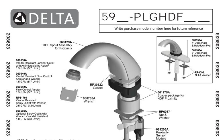
NOTE: For optimum performance of this product, we recommend a system pressure between 20 and 80 PSI static. This product will operate up to a maximum of 125 PSI static per ANSI and CSA requirements. However, we do not recommend pressure above 80 PSI. Thermal expansion or leaking pressure reducing valves may require use of expansion tanks or relief valves to ensure your system never exceeds its maximum intended pressure setting.
