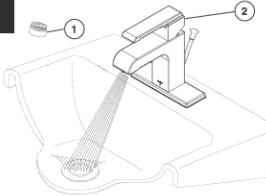
Remove aerator (1) and turn faucet handle (2) all the way on. Turn on hot and cold water supplies (3) and flush water lines for one minute.
