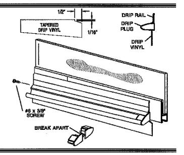
Press the four rail end caps [HH] into the ends of the top and bottom door rails.
