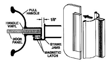
Note: do not use a metal hammer to drive on handle.
