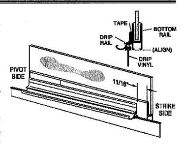
Adjust the drip vinyl [W] by sliding it left or right until it just touches the curb. Trim the vinyl (flush with the pivot end and notch 1/2" longer than the drip rail as shown on the strike end). Secure it with one #6 x 3/8" truss head screw [GG] in the pivot end of the drip rail [U].
