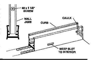
Place the four setting blocks [H] in the curb sembly [A] as shown to support the two fixed glass panels [J]. Position the blocks 3" from the corner of the panels. Set the first glass panel into place on the setting blocks and approximately 1/2" into the wall jamb [E] A strip of masking tape 1/2" from each vertical edge of the glass will aid alignment.
