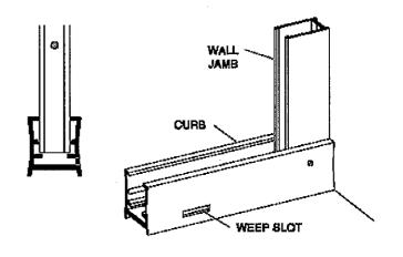
Wipe the shower walls and sill, curb assembly [A] and wall jambs [E] with a clean, dry cloth to remove any dust or debris. Apply a 1/4" bead of caulk along the inside of both of the pencil lines marked in Step #3. Carefully replace the curb in the exact position marked. Caulk the inside of the curb ends where they meet the wall. Caulk generously around the anchor plates [B], screws [C], and the inside of the mitered joints.
