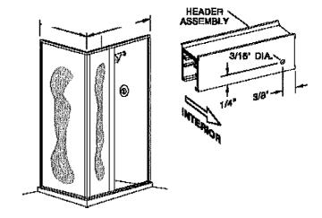
Press the header assembly [D] over the wall jambs [E] 90° post [K] and 180° post [L]. Check the posts for plumb. Adjust as required by varying the overlap of the header over the wall jambs. You may need to trim the ends of the header where it meets the wall. The minimum horizontal dimension for the door opening is the door panel width (see the graphic in Step #9) plus 1/2", maximum is the door panel width plus 1 3/4".
