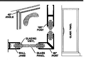
Cut eight pieces of the larger vinyl [LL] 1/2" longer than the horizontal opening and trim the ends on a 45° angle. Install the top exterior vinyl starting at both ends and working toward the middle. Be careful not to stretch the vinyl.
