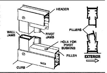
Pull the bottom end of the pivot jamb [N] tight to the curb filler [R] and plumb the jamb. Drill two 1/8" holes thru the pivot jamb and into the wall jamb [E] 3/8" to 3/4" from the wall and approximately 1/4" from the ends of the jamb. Drill a third hole centered between the first two, then enlarge the outer holes with a 3/16" drill for clearance on the self-tapping screws. Attach the pivot jamb permanently with three #8 x 1/4" truss head screws [C].
