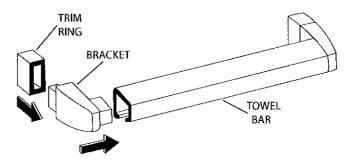
Attach a towel bar assembly (with the open slot in the bar downward) to the interior panel with a #10-24 x 7/8" truss head screw [N] thru the inner rail. Insert a #10-24 x 1 1/8" flat head screw [P] thru an acrylic finger pull [R], thru the outer rail and into the outer towel bar bracket. Peel the backing from a Basco decal [S] press it into the recess in the acrylic finger pull.
