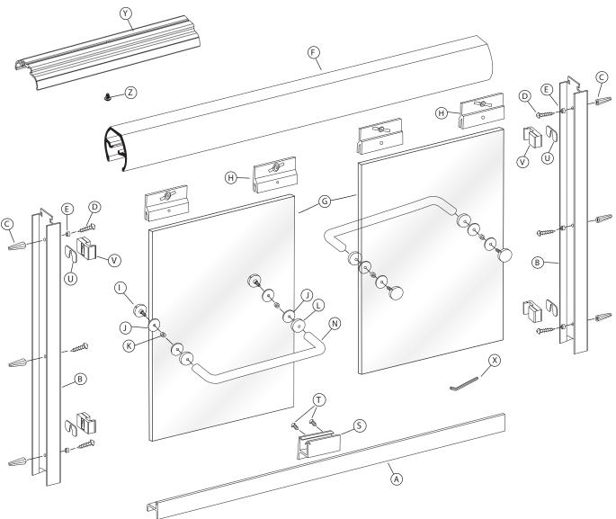
\*\*If installing on a fiberglass unit you may need to snip outside corner to match corners on wall jambs and tub tracks to match radius on fiberglass unit\*\*
