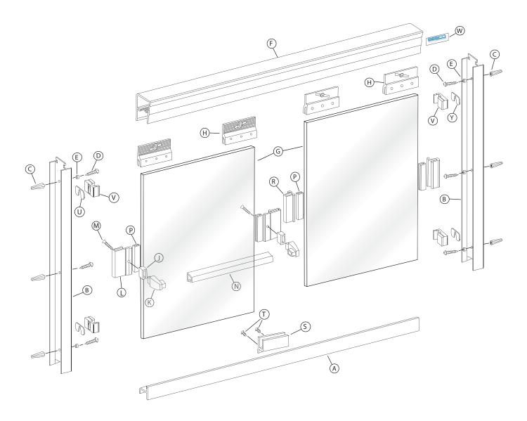
Measure the wall-to-wall opening at the center of the tub rim. Cut the tub track [A] 1/16" short of this dimension. An inexpensive miter box available at your local hardware store will help you get clean square cuts.
