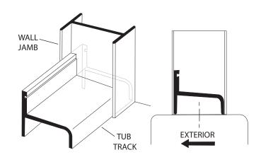
Use a level to plumb both wall jambs [B], then mark the pre-drilled hole locations on the wall. Lightly mark along both sides of the tub track [A] with a pencil, then remove all parts.
