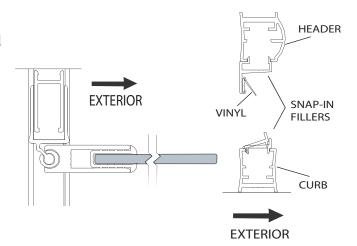
\*\* Prior to installation, be sure that the magnet [N] and vinyl [G] are inserted into the flange. The open part of the vinyl should be facing down and the magnet should be on the side closest to the stationary panel.
