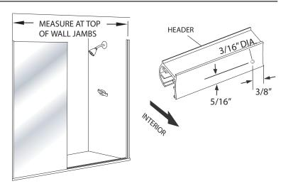
7 Slide the header over the wall jambs. Using the two holes on the interior face of the header as a guide, drill a 1/8" hole into each wall jamb. Attach the header to the wall jambs using two #8 x 1/4" Truss Head screws [H].
