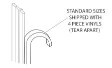
9 Once the panel is set in place, cut four small pieces of the horizontal [J] (crescent shaped) vinyl about 3" and install them into the header and curb (open side of the crescent shape against the glass). This will help hold the panel in place while installing the door panel.
