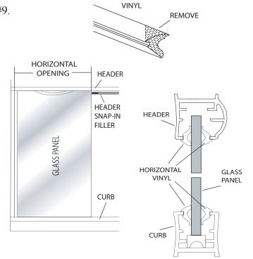
Measure the exposed glass edge of the stationary panel (between top & bottom snap-in fillers).
