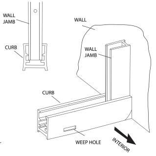
Wipe the shower walls, sill, curb & wall jambs with a clean, dry cloth to remove any dust or debris. Apply a 1/4" bead of silicone along the inside of the pencil lines that were marked in Step #2. Carefully place the curb on the sill, over top the silicone, in the position marked. BE SURE THE WEEP HOLES FACE THE INTERIOR.
