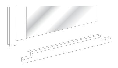
Align the deflector [Q] to the bottom of the door with the hinge side notch over lapping the hinge, then mark the strike side even with the door edge cut deflector at that point.
