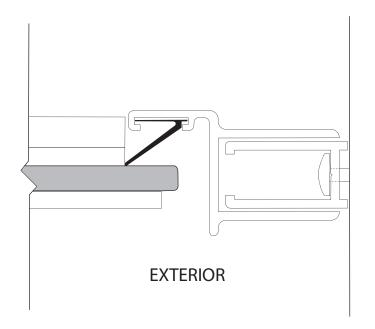
Inspect the pieces of black glazing vinyl, and note the two different profiles. The smaller shape [HH] is installed vertically and the larger shape [JJ] is installed horizontally. For structural strength and maximum water resistance, these vinyls are designed to fit tightly between the glass and framing. To speed installation, use glass cleaner for lubrication and a small block of wood to press the vinyl into place.
