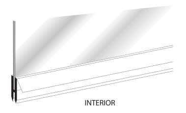
Place the deflector onto the bottom of the door and from inside the shower, close the door and mark the deflector at the edge of the strike jamb. Open the door and remove the deflector. Notch the inside portion of the deflector so the door will close to the strike jamb. Replace the deflector back on the door; close the door to check for clearance.
