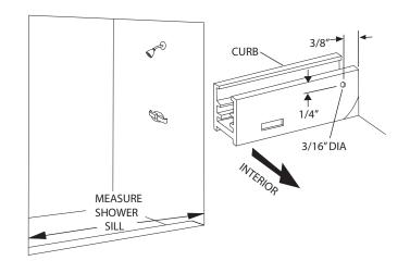
Place the two wall jambs [B] into the ends of the curb [A]. Masking tape may be used to hold the curb in place during this operation. Plumb the jambs and mark the hole locations on the wall. Remove all parts and drill the walls for hardware.
