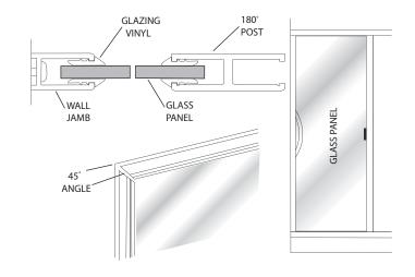
Cut four pieces of the larger vinyl [JJ] 1/2" longer than the horizontal opening and trim the ends on a 45° angle. Install the top exterior vinyl starting at both ends and working toward the middle. Be careful not to stretch the vinyl.
