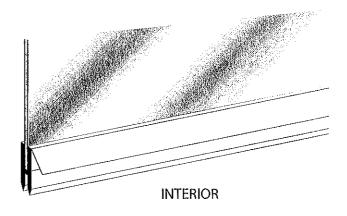
Place the deflector onto the bottom of the door and from inside the shower, close the door and mark the deflector at the edge of the strike jamb. Open the door and remove the deflector. Notch the inside portion of the deflector so the door will close to the strike jamb. Replace the deflector back on the door; close the door to check for clearance.
