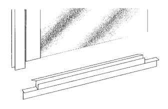
Align the deflector [CC] to the bottom of the door with the hinge side notch over lapping the hinge, then mark the strike side even with the door edge cut deflector at that point.
