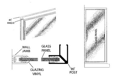
Cut four pieces of the larger vinyl [GG] 1/2" longer than the horizontal opening and trim the ends on a 45° angle. Install the top exterior vinyl starting at both ends and working toward the middle. Be careful not to stretch the vinyl.
