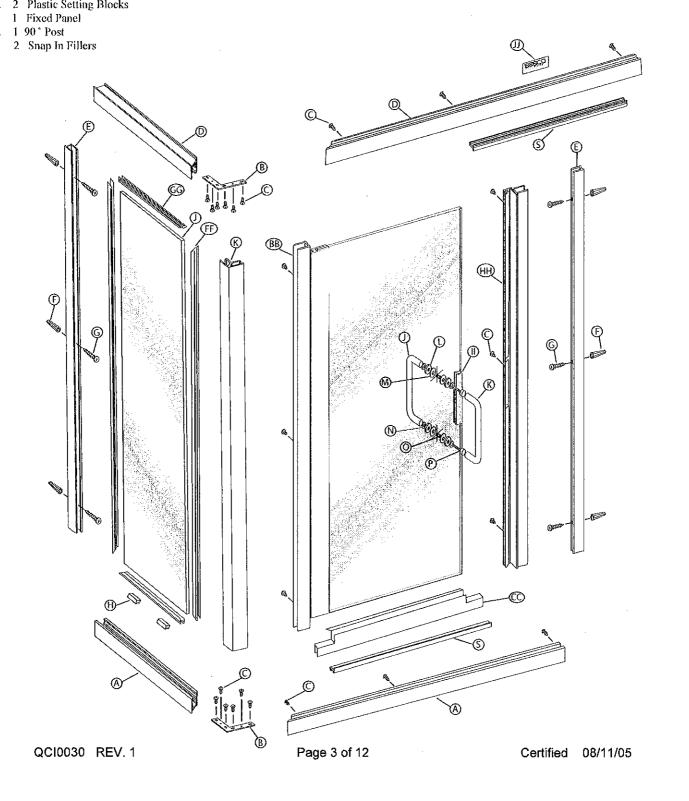
The BASCO 1414/1714 Infinity Shower Door Panel is completely reversible and may be installed hinge-right or hinge-left. The door may hinge from the wall or from the center-post. Using the illustration, determine the correct position for the door in your particular Infinity installation. This instruction sheet depicts a hinge-right installation.
