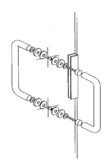
NOTE: The deflector [CC] is notched on both ends. To install deflector, determine if the door is hinge right or hinge left.
