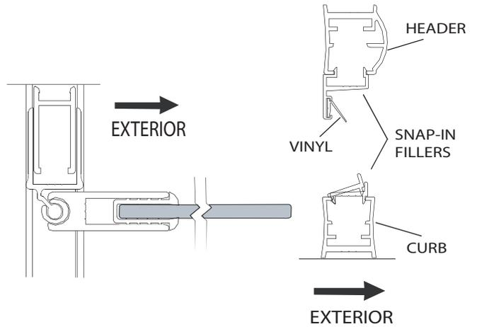
**\*\* Prior to installation, be sure that the magnet [N] and vinyl [G] are inserted into the flange. The open part of the vinyl should be facing down and the magnet should be on the side closest to the stationary panel.**
