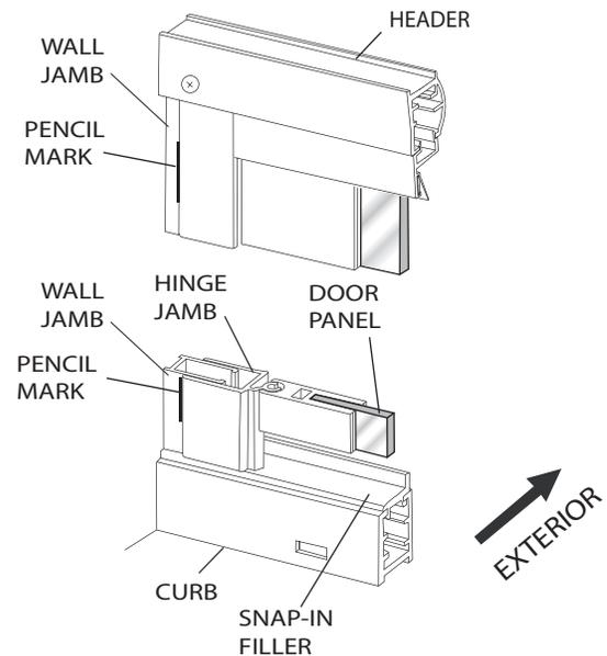
**12** Verify that the door has not shifted using the pencil marks. Then, from the inside of the enclosure, drill two 1/8" holes through the hinge jamb and into the wall jamb approximately 1" from the ends of the jambs at the top and bottom and 3/16" from the edge of the open side of the hinge jamb. (see illustration)
