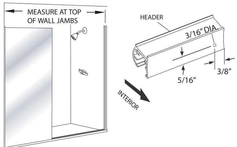
**7** Slide the header over the wall jambs. Using the two holes on the interior face of the header as a guide, drill a 1/8" hole into each wall jamb. Attach the header to the wall jambs using two #8 x 1/4" Truss Head screws [H].
