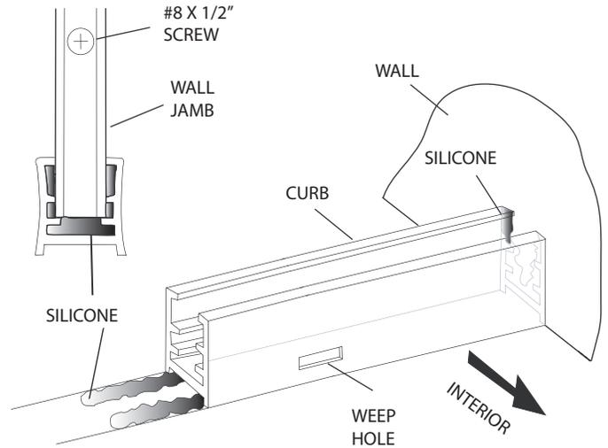
Silicone the inside of the curb at both ends where it meets the wall. **TIP:** Angle the tip so that silicone fills under the two "legs" in the curb that the wall jambs sit on.
