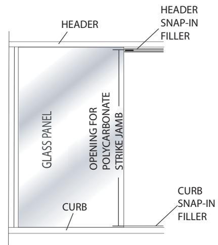
**16** Remove the magnet and slide the vinyl partially out of the header snap-in filler. Trim enough of the vinyl so that the magnet is not covered by the lip of the polycarbonate strike jamb (approximately 3/8" should suffice). Slide the vinyl back into the filler and replace the magnet. Place a small amount of silicone at the end of the magnet to hold in place.
