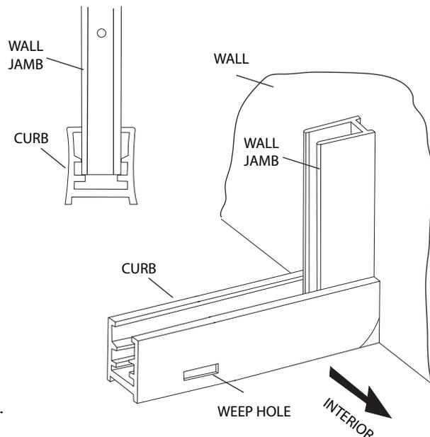
**4** Wipe the shower walls, sill, curb & wall jambs with a clean, dry cloth to remove any dust or debris. Apply a 1/4" bead of silicone along the inside of the pencil lines that were marked in Step #2. Carefully place the curb on the sill, over top the silicone, in the position marked. **BE SURE THE WEEP HOLES FACE THE INTERIOR.**
