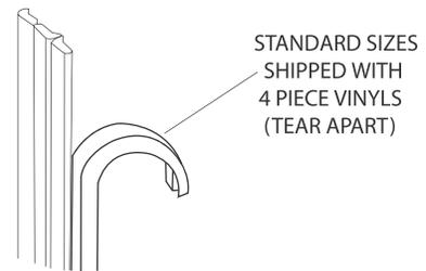
**9** Once the panel is set in place, cut four small pieces of the horizontal [J] (crescent shaped) vinyl about 3" and install them into the header and curb (open side of the crescent shape against the glass). This will help hold the panel in place while installing the door panel.
