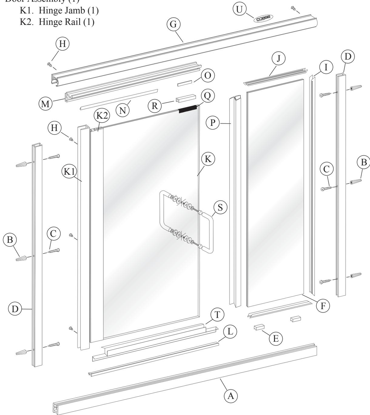
**1** The Basco 1413NP / 1713NP / 1813NP Frameless Continuous Hinge Shower Enclosure must be installed with the door hinged off of the wall. It may be installed hinge right or hinge left. But, for maximum leak protection, the hinge side should be opposite the shower head. Using the illustration, determine the proper hinge side for the door. Careful as to not follow the illustrations exactly.
