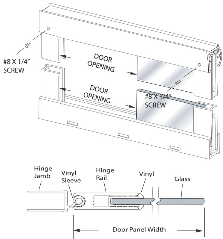
**8** Inspect the strips of black glazing vinyl and note the two different profiles. The flat shaped vinyl [I] is installed vertically and the crescent shaped vinyl [J] is installed horizontally. There should be a minimum of two (2) individual vertical and four (4) individual horizontal pieces of vinyl about a 1/2" wide each. (May need to peel apart from a wider strip).
