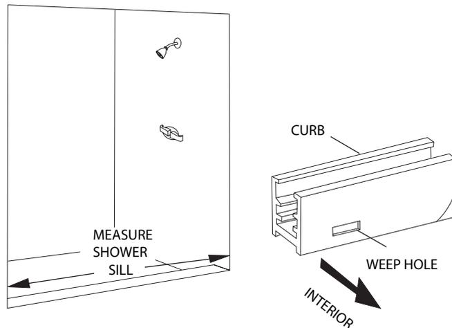
**3** Place one wall jamb [D] into the curb against the wall. Using a level, plumb the wall jamb and mark the hole locations on the wall with a pencil. Repeat this step for the other wall jamb. Remove all parts and drill the holes.
