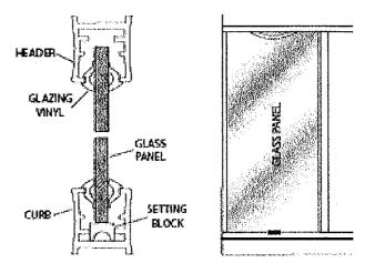
23 Carefully caulk the interior jamb-to-wall and curb-to-base joints. For appearance, you may wish to caulk the exterior joints as well. We recommend you wait twenty-four hours before the first shower to allow the earlking to cure properly.
