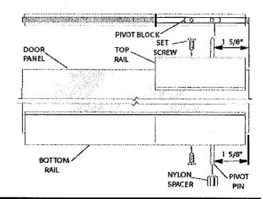
14 Insert the two nylon pivet bushings [AA] into the pivot holes in the head and curb filters [P].
