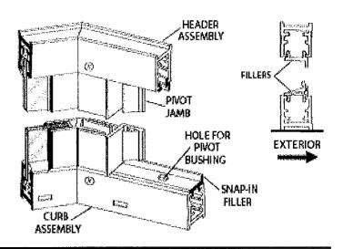
Pull the bottom end of the pivot jamb [M] tight to the carb filler [P] and phunb the jamb, Drill two 1/8" holes thru the pivot jamb and into the 135° post [K] in line with the screws in the head and carb and approximately 1/4" from the ends of the jamb, Drill a third hole centered between the first two, then enlarge the outer holes with a 3/16" drill for eleanance on the self-tapping screws. Attach the pivot jamb permanently with three #8 x 1/4" truss head screws [C].
