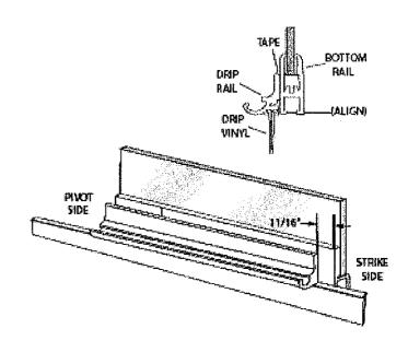
Adjust the drip vinyl [V] by sliding it left or right until it almost touches the carb. Trim the vinyl (flush with the pivot end and notch 1/2" longer than the drip rail as shown on the strike end). Secure it with one #6 x 3/8" truss head serew [FF] in the pivot end of the drip rail [1].
