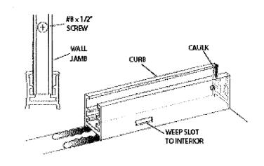
Place the setting blocks [H] in the curb assembly [A] as shown to support the two fixed glass panels [J]. Positioned the blocks 3" from the corner of the panels. Set the first glass panel into place on the setting blocks and approximately 1/2" into the wall jamb [E]. A strip of masking tape 1/2" from each vertical edge of the glass will aid alignment.
