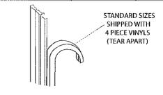
Cut eight pieces of the smaller vinyl [GG] 1" longer than the vertical opening (to prevent gapping from shrinkage) and trim the ends on a  $45^{\circ}$  angle. Using the masking tape guides, center the first glass panel [J] in the frame. Cut four short (1" – 2") pieces of the small vinyl and press into the jamb and post on each side to hold the glass temporarily.
