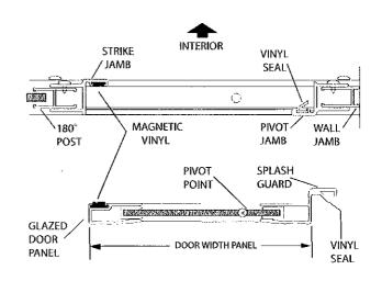
Snap the fillers [R] into the curb assembly [A] and header assembly [D] between the door jambs with the RAISED LIP TO THE EXTERIOR and the pivot holes toward the pivot jamb. Center the curb filler in the curb between the pivot and strike jamb (use masking tape to hold in position).
