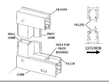
Pull the bottom end of the pivot jamb [P] tight to the curb filler [S] and plumb the jamb. Drill two 1/8" holes thru the pivot jamb and into the wall jamb [E] 3/8" to 3/4"from the wall and approximately 1/4" vertically from the ends of the jamb. Drill a third hole centered between the first two, then enlarge the outer holes with a 3/16" drill for clearance on the self-tapping screws. Attach the pivot jamb permanently with three #8 x 1/4" truss head screws [C].
