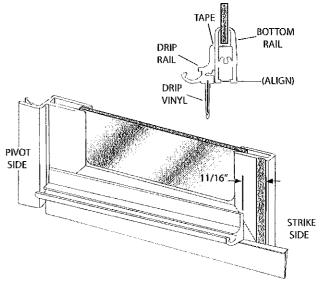
Adjust the drip vinyl [V] by sliding it left or right until it almost touches the curb. Trim the vinyl (flush with the pivot end and notch 1/4" longer than the drip rail as shown on the strike end).
