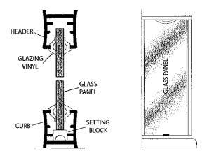
Carefully caulk the interior jamb-to-wall and curb-to-base joints. For appearance, you may wish to caulk the exterior joints as well. We recommend you wait twenty-four hours before the first shower to allow the caulking to cure properly.
