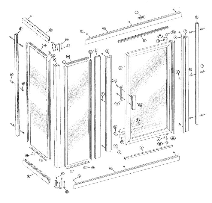
The BASCO 150/750 Thin-Line Shower Enclosure is completely reversible and may be installed pivot-left or pivot-right. The door may pivot from the wall or from the center post. Using the diagram, determine the correct position for the door in your particular Thin-Line installation. This instruction sheet depicts a pivot-right installation.
