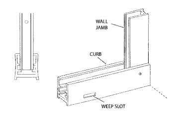
Wipe the shower walls and sill, curb assembly [A] and wall jambs [E] with a clean, dry cloth to remove any dust or debris. Apply a 1/4" bead of caulk along the inside of both of the pencil lines marked in Step #3. Carefully replace the curb in the exact position marked. Caulk the inside of the curb ends where they meet the wall. Caulk generously around the anchor plate [B], screws [C], and the insides of the mitered joint.
