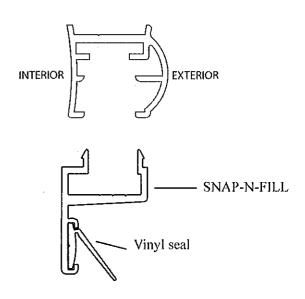
8 Pull the top of the hinge jamb (H) tight with the snap-n-fill (J) use a level to make sure the door panel is plumb.
