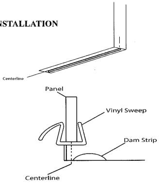
14 Align the deflector to the bottom of the door with the hinge side notch over lapping the hinge, then mark the opposite side even with the door edge cut deflector at that point.
