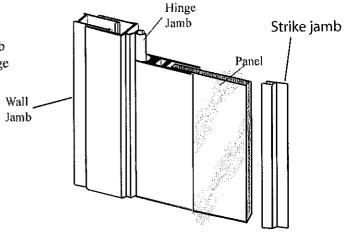
When installing the 2nd panel slide the hinge jamb of the door panel assembly (H) over the mounted wall jamb (B) so the door will open outward while holding the panel, install the snap-n-fill (J) into the header. This will allow you to adjust the 2nd door.
