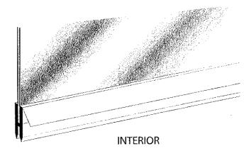
Neatly caulk the inside perimeter of the shower curb and the hinge jamb
