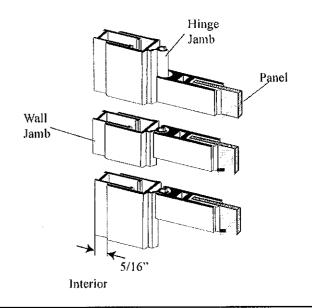
Inside the shower enclosure, drill two 1/8" holes through the hinge jamb and into the wall jamb [B] 3/8" to 3/4" from the wall and approximately 1" vertically from each end of the hinge jamb. Drill a third hole centered between the first two. Attach the door panel assembly permanently with three #6 x 3/8" pan head screws [G].
