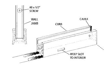
Place the setting blocks [H] in the curb assembly [A] as shown to support the two fixed glass panels [J]. The setting blocks should be positioned approximately 3" from each corner of the panels. Remove any protective strips from the first glass panel and set it into place. It should rest on the setting blocks and be engaged approximately 1/2" into the wall jamb [E]. A strip of masking tape 1/2" from each vertical edge of the glass will aid alignment.
