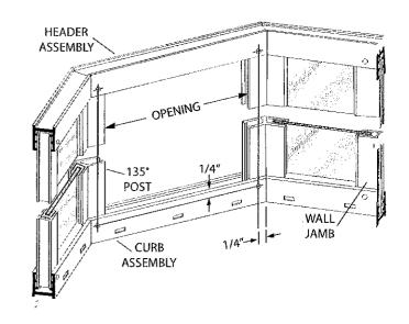
Orient the door to the opening (either hinge right Or hinge left). Place the door in the opening with the door hinge over the wall jamb or post. Carefully hold the door in the opening (in the open position) and don't let go of the door. Place the top filler to the under side of the header WITH THE RAISED LIP TO THE EXTERIOR and snap it into place.
