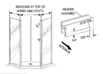
Press the header assembly [D] over the wall jambs [E], the 135° posts [K] and the pre-glazed panels. Check the posts for plumb. Adjust as required by varying the overlap of the header over the wall jambs. You may need to trim the ends of the header where it meets the wall. The minimum horizontal dimension for the door opening is the door panel width (see the graphic in Step #9) plus 1/2", maximum is the door panel width plus 1 3/4".
