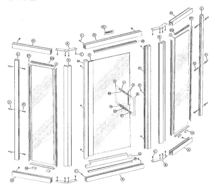
The BASCO 1416 - 1716 Infinity Shower Enclosure is completely reversible and may be installed pivot-left or pivot-right. For maximum waterproofing, the pivot jamb should be opposite the shower head. Using the diagram, determine the correct position for the door in your particular Quick-N-Stall installation. This instruction sheet depicts a pivot-right installation.
