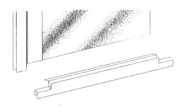
Align the deflector [U] to the bottom of the door with the hinge side notch over lapping the hinge, then mark the strike side even with the door edge cut deflector at that point.
