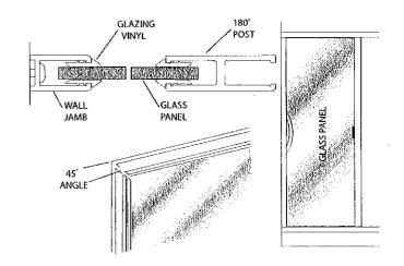
Cut eight pieces of the larger vinyl [JJ] 1/2" longer than the horizontal opening and trim the ends on a 45° angle. Install the top exterior vinyl starting at both ends and working toward the middle. Be careful not to stretch the vinyl.
