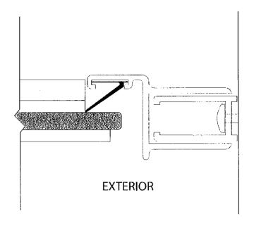
Inspect the pieces of black glazing vinyl, and note the two different profiles. The smaller shape [HH] is installed vertically and the larger shape [JJ] is installed horizontally. For structural strength and maximum water resistance, these vinyls are designed to fit tightly between the glass and framing. To speed installation, use glass cleaner for lubrication and a small block of wood to press the vinyl into place.
