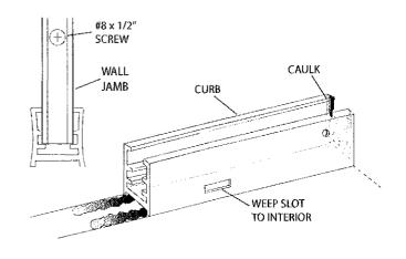
Place two setting blocks [E] into the curb [A] to support the fixed glass panel [F]. Position the blocks 3" from each corner of the glass panel. Set the glass panel into place on the setting blocks and approximately 1/2" into the wall jamb [B]. A strip of masking tape 1/2" from each vertical edge of the glass will aid alignment. Repeat for second panel.
