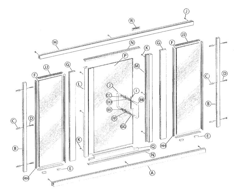
The BASCO 1412/1712 Continuous Hinge Shower Enclosure is completely reversible and may be installed swing-right or swing-left. The door may hinge from the glass or from the center-post. For maximum waterproofing, the hinge jamb should always be opposite the shower head. Using the illustration, determine the correct position for the door in your particular Infinity installation. This instruction sheet depicts a hinge-right installation.
