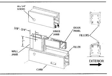
Pull the bottom end of the hinge jamb [L] tight to the curb filler [N] and plumb the jamb. Drill two 1/8" holes thru the hinge jamb and into the wall jamb [B] 3/8" to 3/4" from the wall and approximately 1/4" from the ends of the jamb. Drill a third hole centered between the first two, then enlarge the three outer holes with a 3/16" drill for clearance on the self-tapping screws. Attach the pivot jamb permanently with three #8 x 1/4" truss head screws [K].
