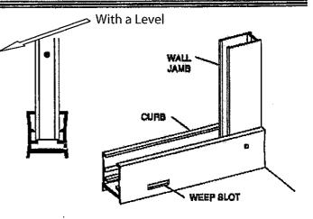
Wipe the shower walls and sill, curb [A] and wall jambs [B] with a clean, dry cloth to remove any dust or debris. Apply a 1/4" bead of caulk along the inside of both of the pencil lines marked in Step #2. Carefully replace the curb in the exact position marked. Caulk the inside of the curb where it meets the wall.
