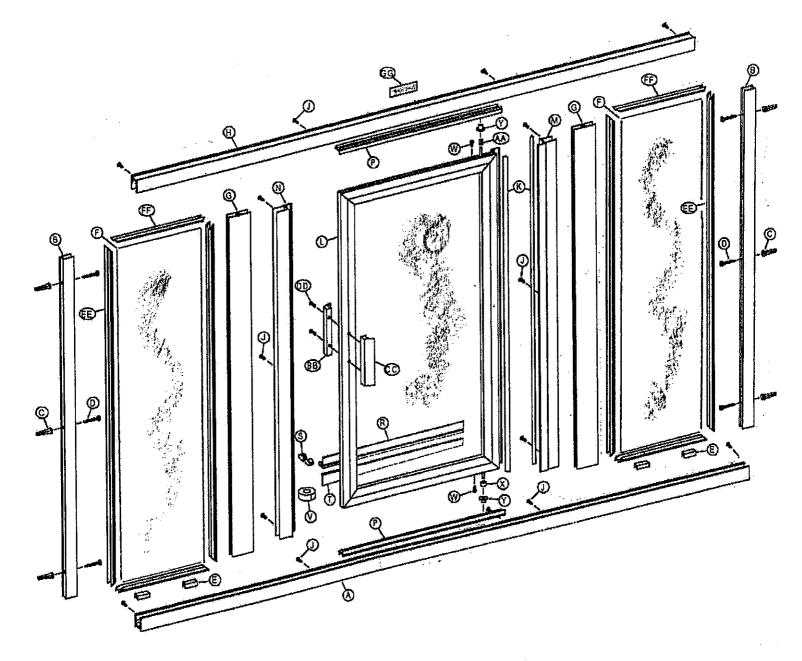
The BASCO 125S/125/725 Thin-Line Shower Enclosure is completely reversible and may be installed pivot-left or pivot-right. The door may pivot from the wall or from either center post. For maximum waterproofing, the pivot jamb should be opposite the showerhead. Using the diagram, to determine the correct position for the door in your particular installation. This instruction sheet depicts a pivot-right installation.
