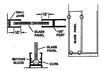
Measure the wall-to-wall opening at the top of the wall jambs [B] and cut the header [H] to fit the exact opening. Using a 3/16" drill bit, drill the interior face of the header on both ends as shown.
