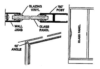
Cut four pieces of the larger vinyl [FF] 1/2" longer than the horizontal opening and trim the ends on a 45° angle. Install the top exterior vinyl starting at both ends and working toward the middle. Be careful not to stretch the vinyl.
