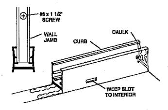
Place the setting blocks [E] in the curb [A] as shown to support the fixed glass panel [F]. The setting blocks should be positioned approximately 3" from each corner of the glass panel. Remove any protective strips from the glass panel and set it into place. It should rest on the setting blocks and be engaged approximately 1/2" into the wall jamb [B]. A strip a masking tape 1/2" from each vertical edge of the glass will aid alignment.
