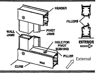
Pull the bottom of the pivot jamb [M] tight to the curb filler [P] and plumb the jamb. Drill two 1/8" holes thru the pivot jamb and into the 180 degree post [G] 3/8" to 3/4" from the wall and approximately 1/4" vertically from the ends of the jamb. Drill a third hole centered between the first two and enlarge the outer holes with a 3/16" drill for clearance on the self-tapping screws. Attach the pivot jamb permanently with three #8 x 1/4" truss head screws [J].
