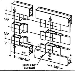
Clean the bottom door rail and the drip rail thoroughly with rubbing alcohol to ensure proper adhesion. Unroll the double stick tape [V] and carefully apply it to the back of the drip rail (do not peel the tape backing yet).
