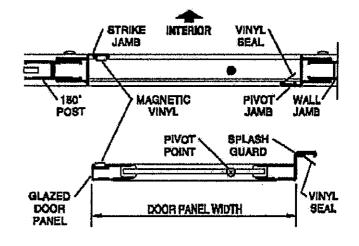
Snap the fillers [P] into the curb [A] and header [H] between the door jambs with the RAISED LIP TO THE EXTERIOR exterior and the pivot holes toward the pivot jamb. Center the curb filler in the curb between the pivot and strike jamb (use masking tape to hold in position).
