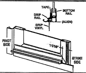
Adjust the drip vinyl [T] by sliding it left or right until it just touches the curb. Trim the vinyl (flush with the pivot end and notch 1/4" longer than the drip rail as shown on the strike end).
