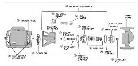
The best way to repair a pump is to order a **Bearing Assembly**. It includes all the component parts preassembled into an easy-to-install pump housing.
