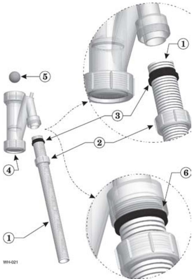
Figure 48 Condensate trap assembly into jacket
