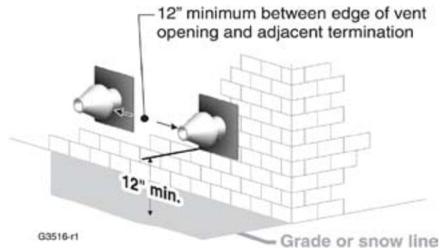
**Figure 27** Installing and supporting the concentric sidewall vent assembly
