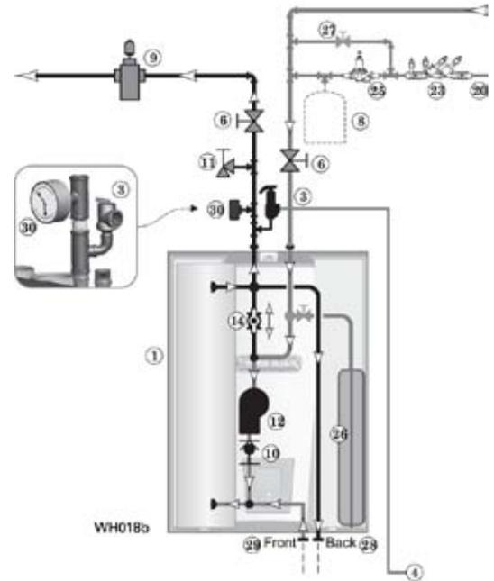
**Figure 38** External expansion tank piping, closed-type expansion tank
