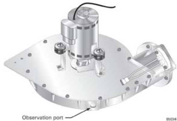
Figure 78 Igniter observation port in blower
