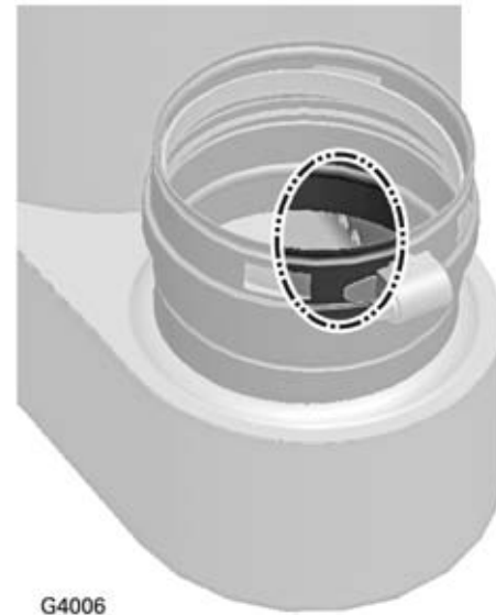
Figure 84 Recuperator flueway drain holes
