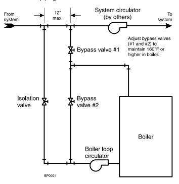
Figure 17 Boiler bypass piping — use only for high water content systems —DO NOT use for radiant panel systems.
