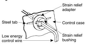
Figure 26 Connect field wiring in boiler junction box as shown below. See Control Supplement for more details.
