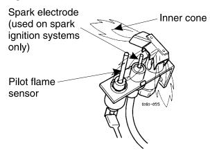
Figure 29 Typical main burner flame
