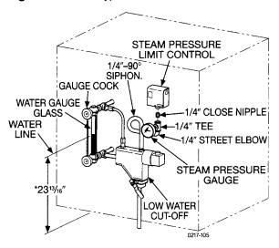
Figure 23 Piping for optional float-type water level controllers for steam boilers
