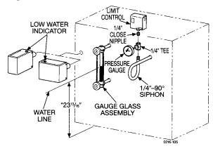
Figure 22 Float-type low water cut-off
