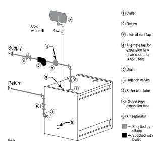
Figure 14 Recommended piping – forced hot water boilers with diaphragm type expansion tanks
