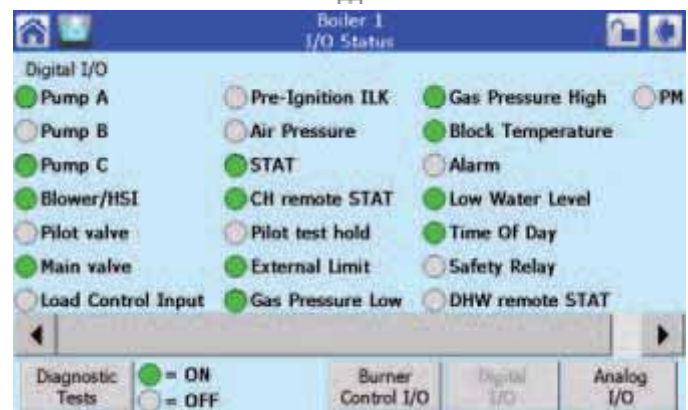
Figure 70 Digital I/O Status page (HOME PAGE → → DIAGNOSTICS)
