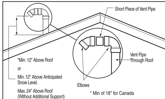
Figure 6 – Vertical Vent Terminal Location
