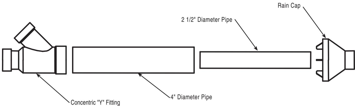
**Figure 14. - Concentric Vent Kit Part Identification**
