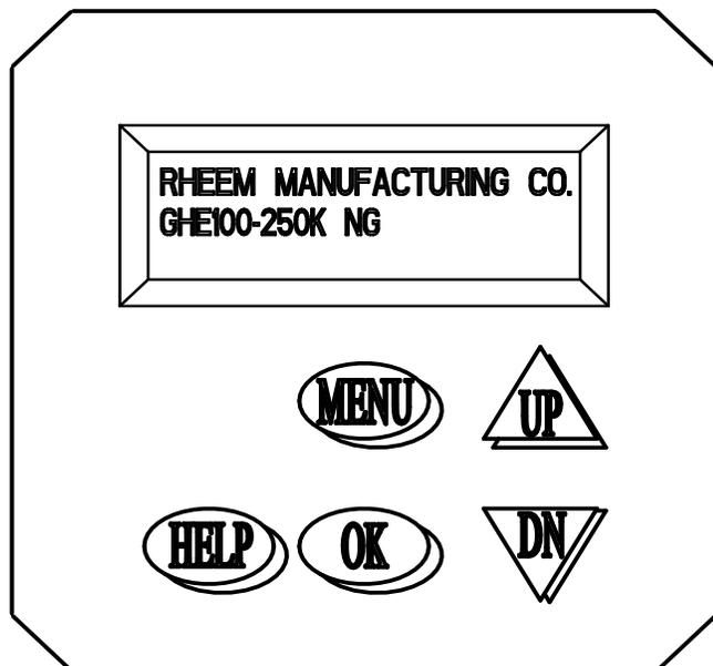
If the screen on the display is flashing, the burner did not light. To reset the ignition sequence, press the "HELP" button and then the "OK" button (see Display screen at left). On initial startup, it might be necessary to clear the "flashing" screen two or three times, to make sure that the gas has made its way to the burner. If the unit has been operating and then shows the flashing display, then there is another issue to be resolved (unless gas has been off).
