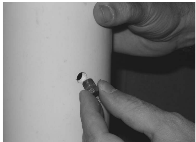
Figure 9.3: Insert Pipe Plug into Test Port
