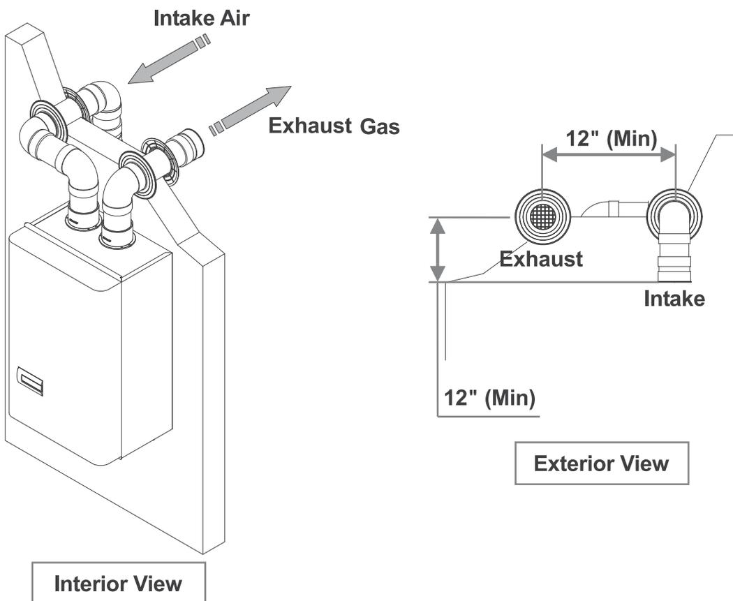
**Option #2:** Non-concentric venting through a side wall. Air is drawn from different location at a **minimum** of 12" from the termination. Please try to minimize the length of the intake air pipe length.
