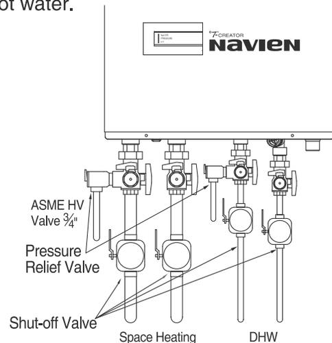
Instructions for pressure, temperature and vacuum relief valves shall specify that no valve is to be placed between the relief valve and the tank. The instructions shall specify installation in such a manner that the discharge from temperature and pressure relief valves will be conducted to a suitable place for disposal when relief occurs and that no reducing coupling or other restriction be installed in the discharge line.
