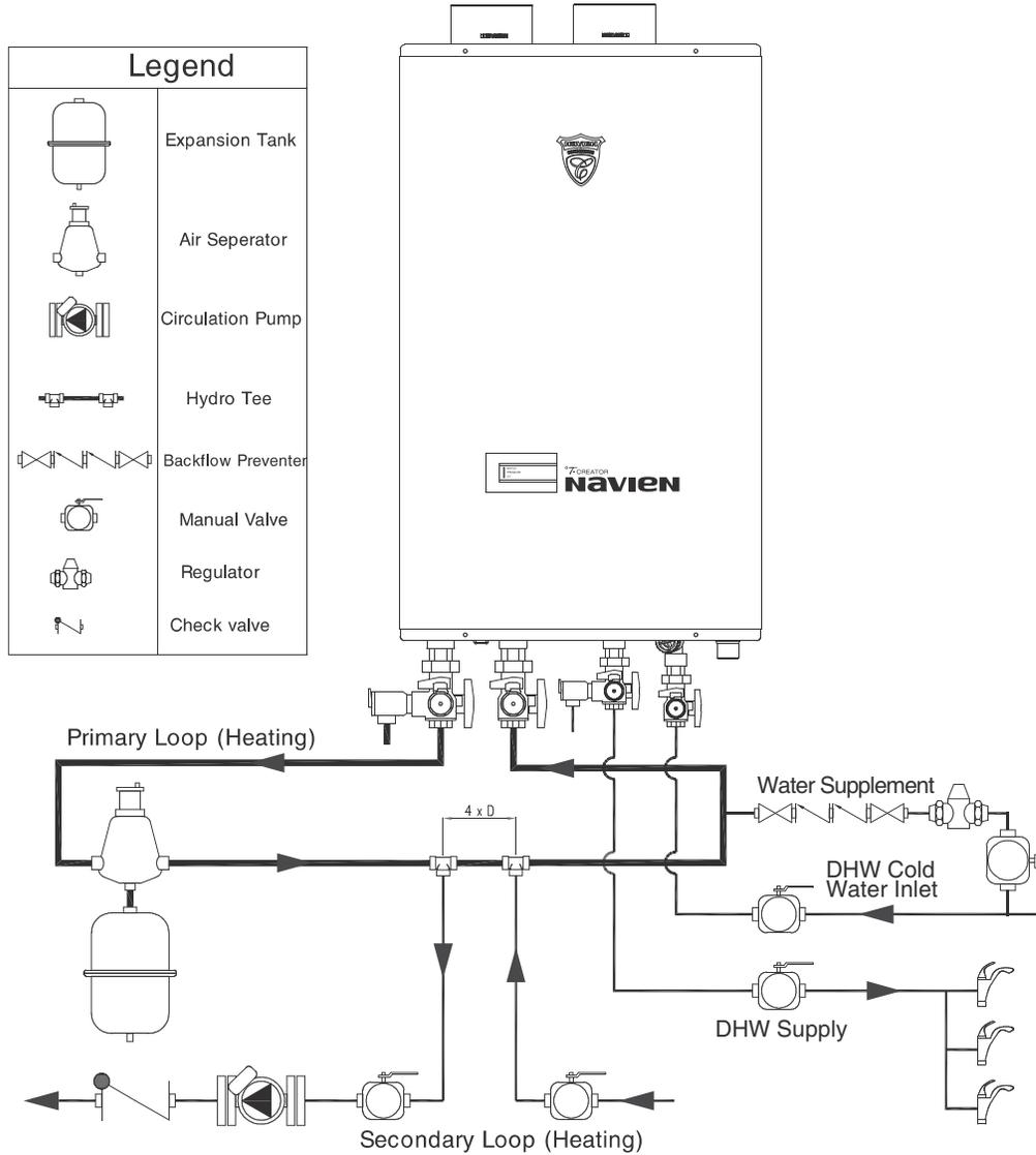
As shown above, Navien's have to establish the water supplement plumbing is not recommended.
