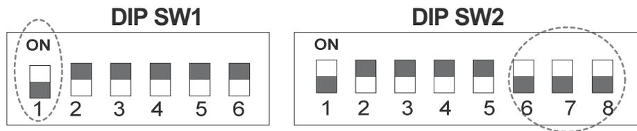
DIP Switch set-up of the master unit PCB: Slave unit addition/removal
