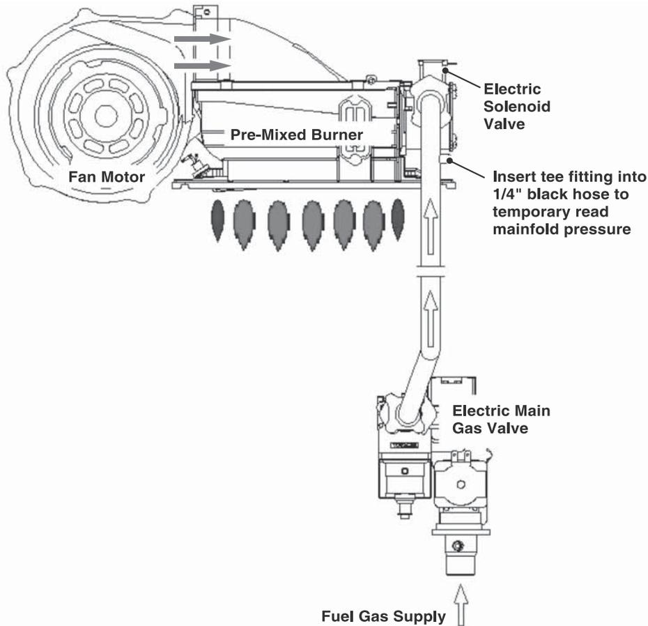
The Navien Combination Boiler cannot operate properly without sufficient inlet gas pressure and volume. Below are instructions on how to check the inlet gas pressure.
