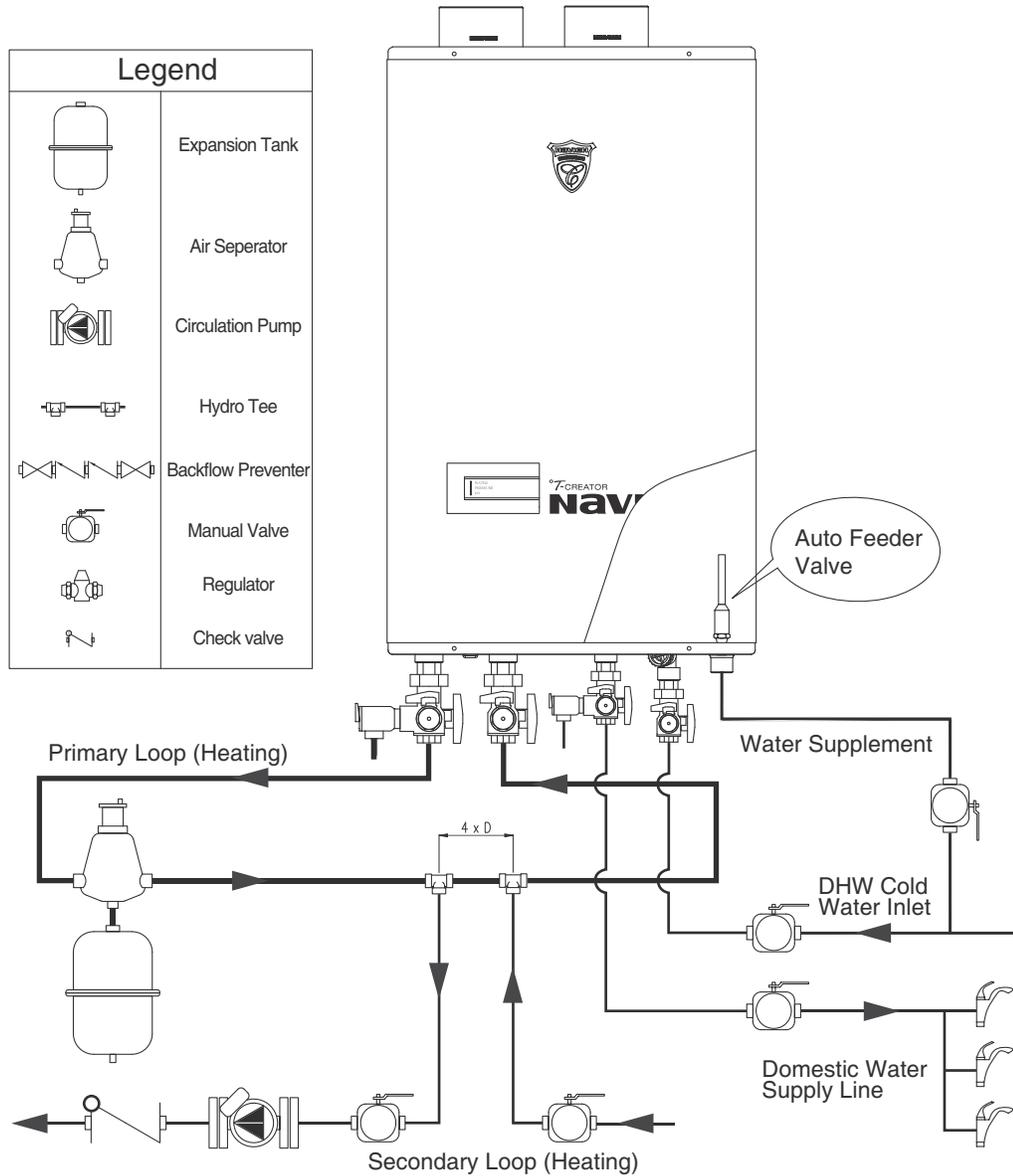
**NOTICE :** If using mixing valves on the domestic hot water outlet, choose one which prevents cold water pressure from overcoming hot water line pressure. Hot water Temperature may vary when more than two faucets (appliances, fixtures, etc.) are being used simultaneously.
