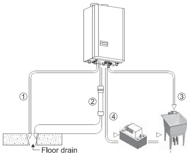
**Note:** Do not cap(or plug) the intergrated condensate line. Without proper drainage or disposal, condensate will damage the Navien Boiler.
