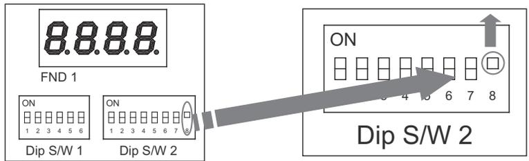
[DIP Switch Setting of High Temperature Applications]
