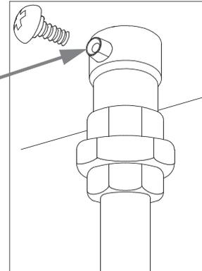
4. Connect a manometer to the pressure port and reset it to zero.
