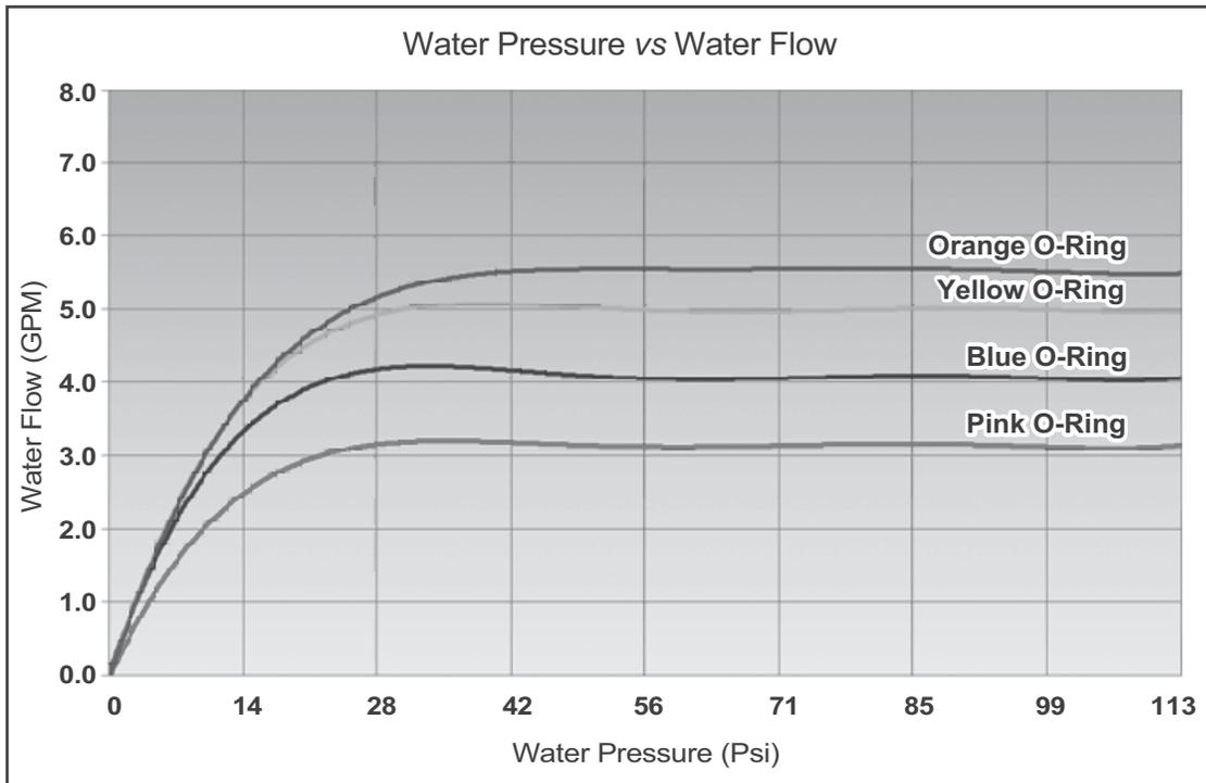
See graph above for the water flow(GPM) and water pressure(psi) to install the pressure reducing valve.
