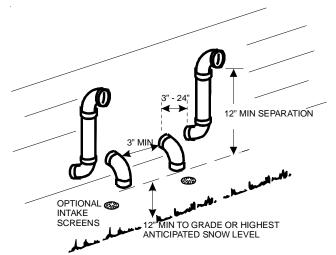
Termination of Multiple Direct Vent Furnaces Figure 19
