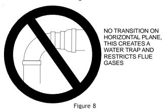
Precautions should be taken to prevent condensate from freezing inside the vent/flue pipe and/or at the vent/flue pipe termination. All vent/flue piping exposed to temperatures below 35°F for extended periods of time must be insulated with 1/2" thick closed cell foam. Also, all vent/flue piping exposed outdoors in excess of the terminations shown in this manual (or in unheated areas) must be insulated with 1/2" thick closed cell foam. Inspect piping for leaks prior to installing insulation.
