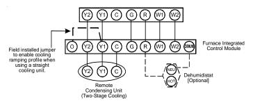
Thermostat - Two-Stage Heating with Two-Stage Cooling Figure 33
