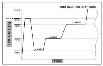
Operation with Conventional 1-Stage Thermostat (DIP switch selects 1-Stage heat) Figure 44
