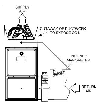
Checking Static Pressure Figure 40
