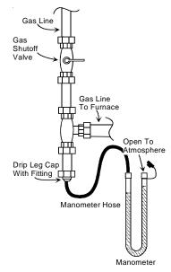
Measuring Inlet Gas Pressure (Alt. Method) Figure 50
