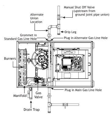
Drip leg may terminate with a 1/2" x 1/8" pipe plug to accommodate line gas pressure measurement.
