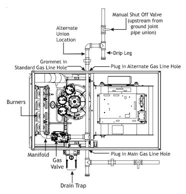
When gas line is in the alternate location, swap the position of the plug and grommet.
