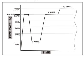
Operation with Conventional 2-Stage Thermostat (DIP switch selects 2-stage heat) Figure 46
