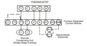
Thermostat - Single-Stage Heating with Single-Stage Cooling Figure 31
