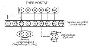
Thermostat - Two-Stage Heating with Single-Stage Cooling Figure 32
