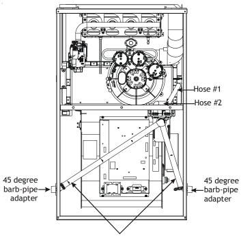
Installer selects right or left side drain and installs this hose accordingly.
