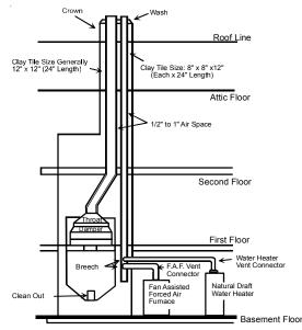
Typical Multiple Flue Clay Tile Chimney
