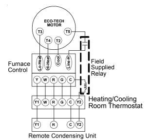
Field Wiring for GME8 Furnace with 2-Stage Condenser
