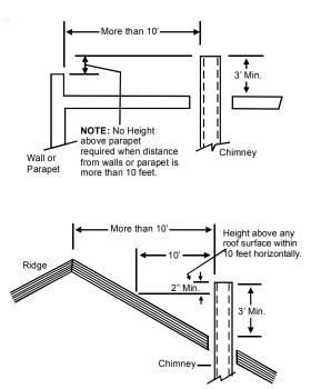
Termination More Than 10 Feet From Ridge, Wall or Parapet
