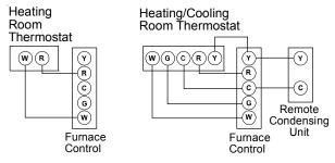
Typical Field Wiring (24 VAC Control Circuit)
