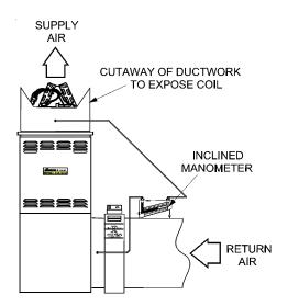
Checking Static Pressure (80% Furnace Shown, 90% Similar)
