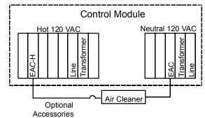
If it is necessary for the installer to supply additional line voltage wiring to the inside of the furnace, the wiring must conform to all local codes, and have a minimum temperature rating of 105°C. All line voltage wire splices must be made inside the furnace junction box.
