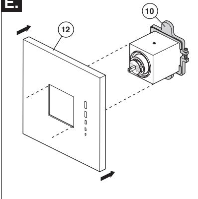
Place the center hole of the escutcheon (12) over the trim sleeve and carefully push it back to the mounting plates (10). Magnets on the back of the escutcheon will keep it in place.
