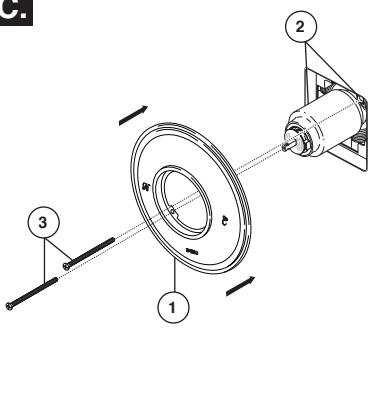
Secure the escutcheon (1) to the bracket (2) using the 2 screws provided (3). Do not overtighten escutcheon screws.
