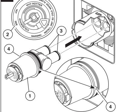
Rotate the cartridge (1) so the words “hot side” (2) appear on the left. Insert cartridge into valve body as shown. Make sure the cartridge tubes and O-rings (3) are properly seated in holes at the base of the body. Ensure the keys on the body are fully engaged with the slots in the body (4).
