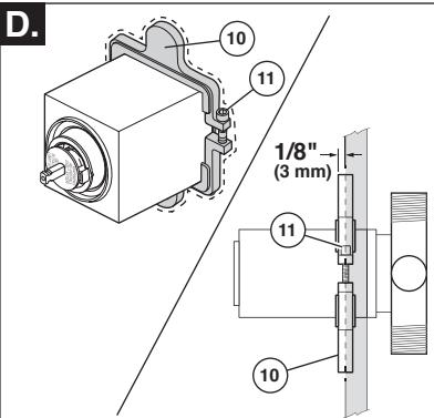
Using the mounting plates (10) as a guide, enlarge hole around rough so that plates can be pushed up to  $1/8"$  into the wall. Tighten screws (11).
