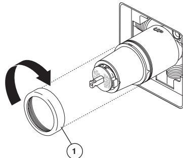
Slide bonnet nut (1) over the cartridge and thread onto the body. Hand tighten securely.
