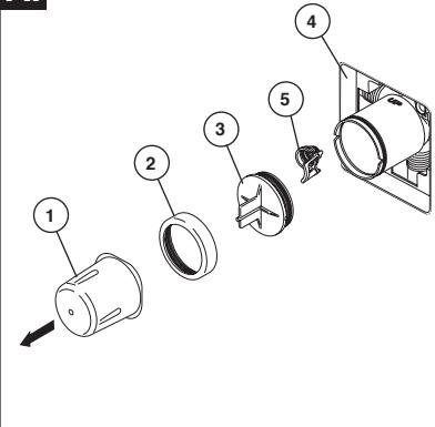
**Turn off water supplies.** Remove cover (1), bonnet nut (2) and test cap (3) from the body. If this is not a thin wall mounting, the entire plastrugard (4) may be removed. If screen (5) is in place, remove before installing cartridge.
