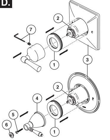
Slide trim ring (1) over trim sleeve (2) and insert into escutcheon (3). **Models T60P210 & T60P410** - Secure handle (4) onto the stem using screw (5) and a phillips head screwdriver. Insert button (6) into handle. **Other models** - Secure handle onto the stem using set screw and Allen wrench (7).
