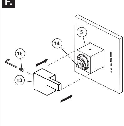
Place handle (13) over valve stem (14) and onto the trim sleeve (5). Lever should point horizontally to 3 o'clock position. Secure handle with set screw (15).
