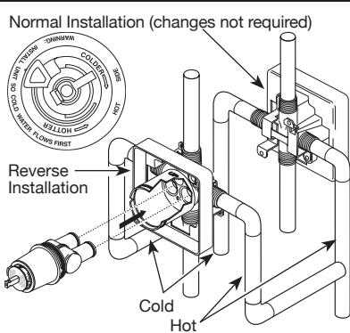
For back to back or reverse installations (hot on right and cold on left) insert the cartridge with the “hot side” on the right. If you are not making a reverse or back to back installation skip this step and continue with step 1C.
