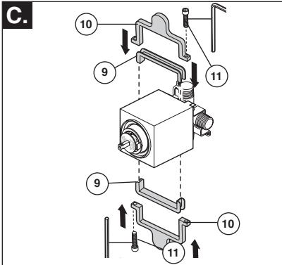
Assemble the two mounting sleeves (9) and two mounting plates (10). Slide the mounting plate assemblies over the trim sleeve so that the tabs/plates (10) are at the top and bottom of the trim sleeve, as shown. Thread screws (11) into mounting plates just enough to assemble the two sides together. Slide the mounting plates back against the wall and finish tightening the screws (11).
