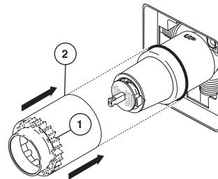
Slide O-ring (1) over cartridge and the bonnet nut (2). The O-ring, which acts as a spacer to steady the sleeve, should rest behind the bonnet nut.
