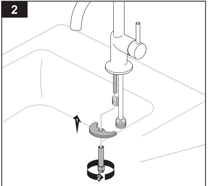
Slide metal bracket over mounting stud under sink. Secure with mounting nut. Tighten securely but do not over tighten.
