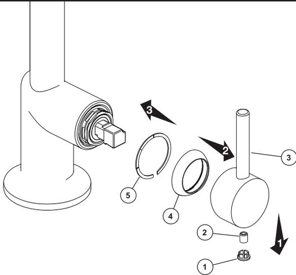
Add optional temperature ring by removing button (1), set screw (2), handle (3) and bonnet (4). Install temperature ring (5), ensure that ring is aligned with the open notch on faucet. When reinstalling parts, make sure bonnet cap is pressed on securely.
