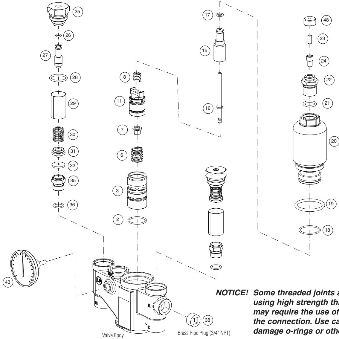
**NOTICE!** Some threaded joints are assembled using high strength thread lock and may require the use of heat to loosen the connection. Use caution to not damage o-rings or other components.
