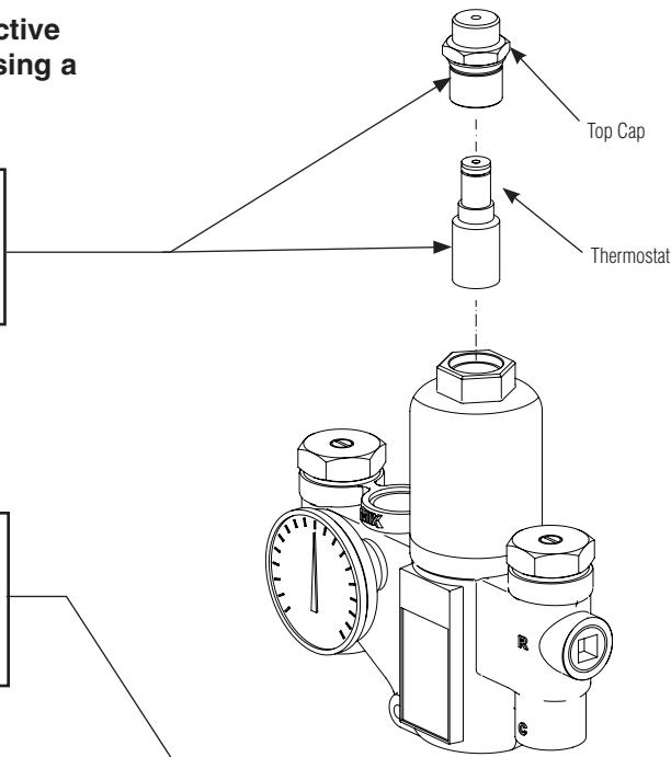
**B** Insert a 7/16" dia. rod into the valve until it touches the top of the pushrod that is attached to the piston. Mark the length of the rod inside the valve. Push the rod until the piston stops and mark the new length.
