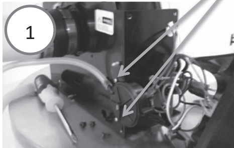
Remove 3 Phillips screws to remove cover.
