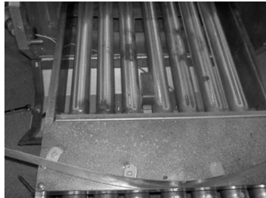
Step 14: Slide out burner assembly
