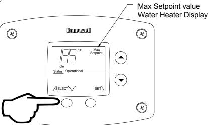
2a. Water Temperature Average (Displays average if there are two sensors – sensor temperature displayed if single sensor is used).
