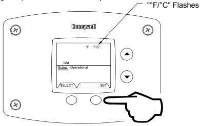
Step 3a: Press "Temperature Up" button to change temperature format to °C
