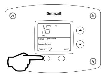
3. Flame Current of Pilot Flame Sensor (Displays only in the Heating Cycle)
