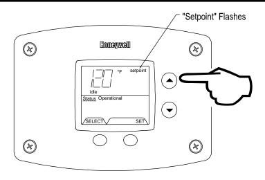
Step 4: To lower the temperature setpoint, press the "Temperature Down" button until the desired temperature is shown on the water heater display.
