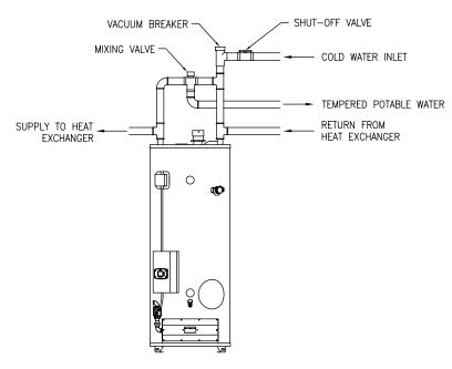
Suggested Piping Arrangement For Top Connections
