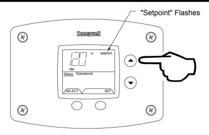
Step 4: To lower the temperature setpoint, press the "Temperature Down" button until the desired temperature is shown on the water heater display.
