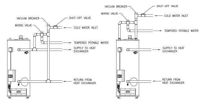
Suggested Piping Arrangement For Side Connections Suggested Piping Arrangement For Top and Side Connections
