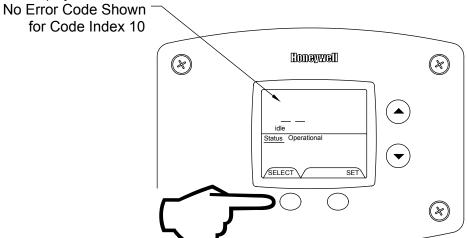
Step 4: Press the "Temperature Down" button to change to the previous code index, code #9.
