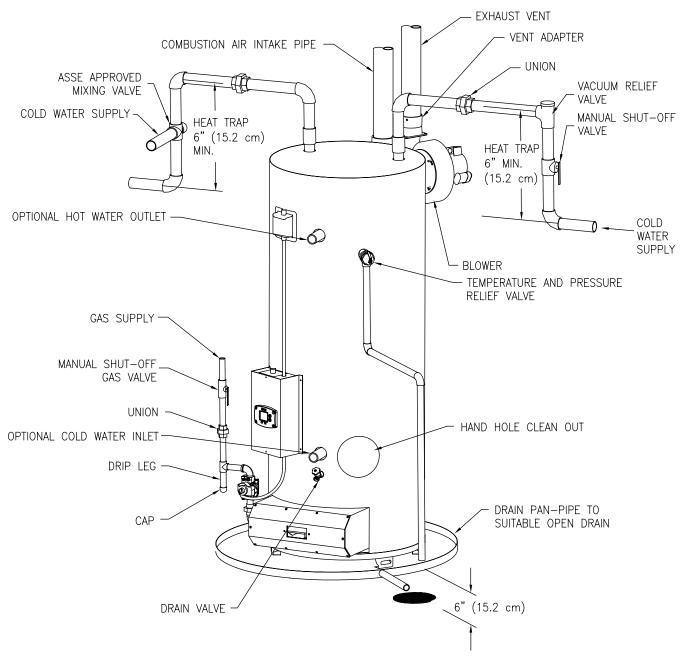
Notes: The heat trap shown above is not part of the water heater, only a piping suggestion to reduce the standby heat loss. The drain pan may be purchased from your water heater supplier.
