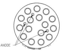
FRONT OF WATER HEATER INDUCED DRAFT MODELS (D80T725, D65T625)
