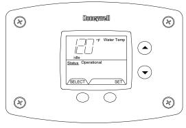
2b. Water Temperature - Upper Sensor (Displays if there is an upper sensor - some models)
