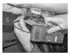
Checking pressure switch contacts.
