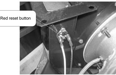
Vent safety thermal switch on PDV-S blower. Depress red reset button in center of switch. If a slight click is felt, switch opened. Check for loose or leaking burner access panel (see section on servicing burners)
