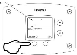
Step 2: Press the "Temperature Down" button to select the error code index, starting with the most recent error code "10".
