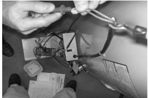
Checking continuity of upper sensor wire harness.
