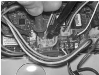
Checking MV pin terminal to gas valve wire harness for 24 volts output to gas valve during heating cycle (pilot must be lit with no sparking).
