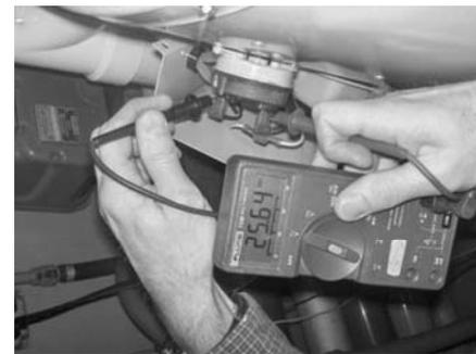
Checking pressure switch contacts. Contacts are open if blower is operating and there is 22-26 volts measured between the two contacts (as in photos)
