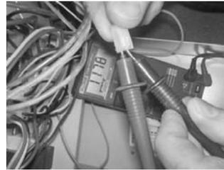
Checking resistance of lower sensor (center and outside pins)
