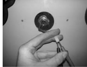
Checking resistance of upper sensor
