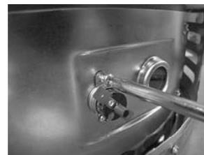
Step 5. Place new resettable thermal switch in place. Be sure contact surface of resettable thermal switch and inner door are free of any debris. Secure resettable thermal switch into place using screws from step 4. **DO NOT OVER TIGHTEN SCREWS.**
