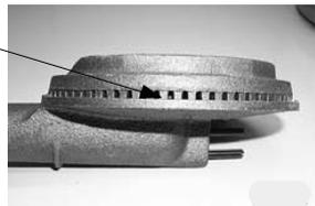
Step 4. On cast iron burners, inspect for any debris build up inside burner venturi. If found, disconnect feedline from burner and remove debris build up.
