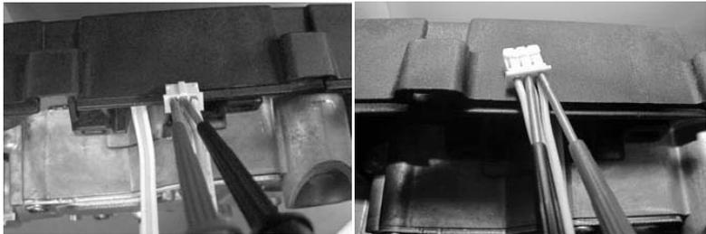
Using a multi-meter set to the ohms setting, insert one meter probe (see caution) into center wire position of thermal well connector, insert the second probe (see caution) into either of the outside wire positions (see photo on left).
