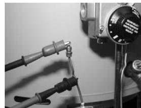
Step 3. Following the lighting instruction label on the heater, proceed to light the pilot and allow to operate for three minutes. **It will be necessary to hold the pilot button down continuously throughout this test.** A reading of 20 to 30 millivolts indicates good thermocouple output.
