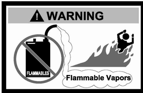
Water heaters are heat producing appliances. To avoid damage or injury there shall be no materials stored against the water heater or vent-air intake system, and proper care shall be taken to avoid unnecessary contact (especially by children) with the water heater and vent-air intake system.
