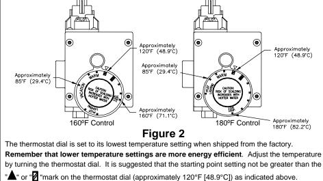
Rotate the thermostat dial **clockwise** to <u>decrease</u> the temperature setting. Rotate the thermostat dial **counter-clockwise** to <u>increase</u> the temperature setting. Adjust the dial until the minimum acceptable temperature is achieved (See figure 2 above for approximate temperature settings).
