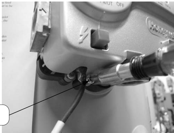
Rotate knob counter-clockwise to the “OFF” position.
