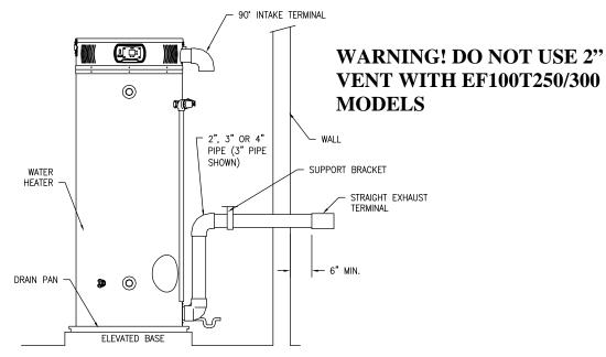
Figure 15. Typical Horizontal Power Vent System
