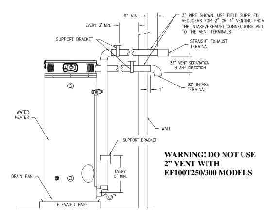
Figure 12. Typical Horizontal Direct Vent System
