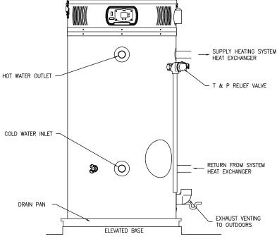
Figure 9. Alternate Space Heating Connections
