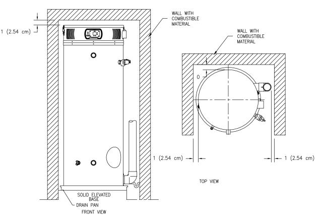
Figure 3a. Minimum Clearance To Combustible Material
