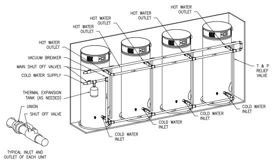
Figure 8. Typical Four Water Heater Connection
