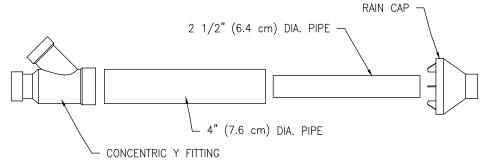
Figure 20. Concentric Vent Kit Part Identification
