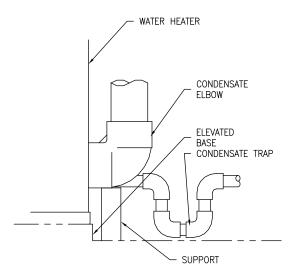
Figure 2. Condensate Elbow With Trap
