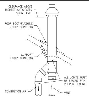
Figure 22. Concentric Vent Roof Top Attachment
