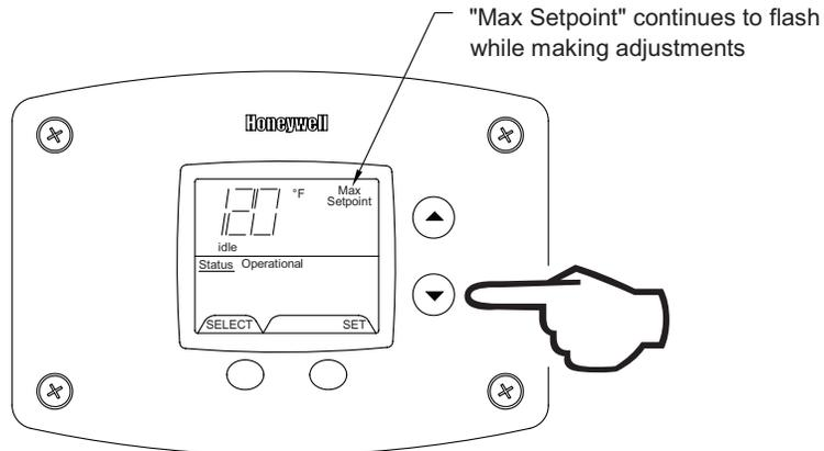
Step 4: Press "Set" button to confirm new "Max Setpoint" value and stop setting mode.
