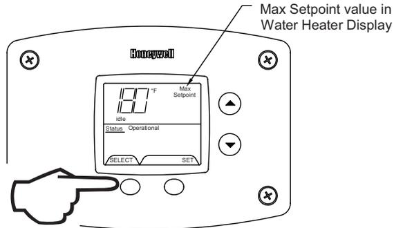
2. Tank Sensor Temperature Displayed Water Temperature Average.
