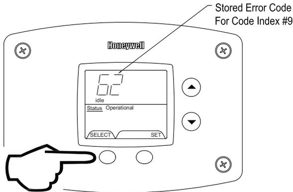
Step 6: Continue pressing the “Temperature Down” button to change to the next error code index and press “Select” to view the error code number, if any, for that index number. Continue on to index #1, the oldest error code index. The water heater display will store up to 10 error codes with the oldest code starting in code index #1 with the most recent code in code index #10.
