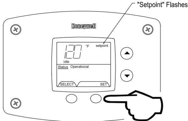
Step 3: To raise the temperature setpoint, press the "Temperature Up" button until the desired temperature is shown on the water heater display.
