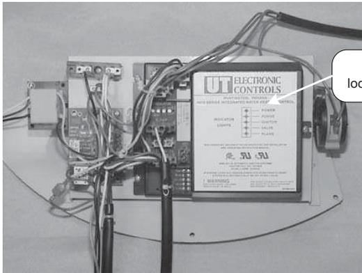
**Note: Replacement hot surface ignition module works on all EF models prior to and later than "CF" serial numbers. Direct spark ignition models use a different control board (detailed in following section).**
