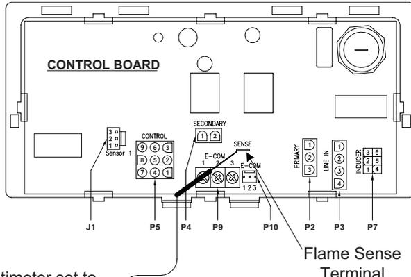
Multimeter set to microamp (µA) setting
