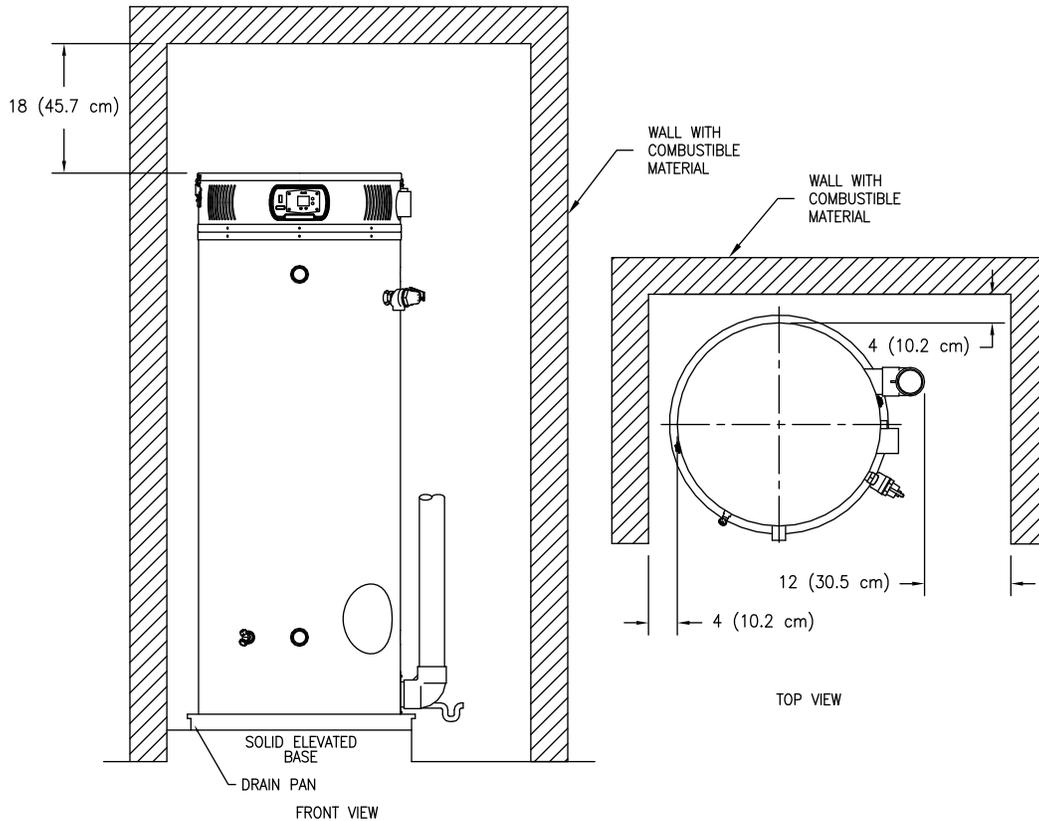
**Figure 3b. Recommended Minimum Clearances For Service Access**
