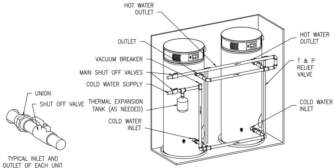
Figure 6. Typical Two Water Heater Connection
