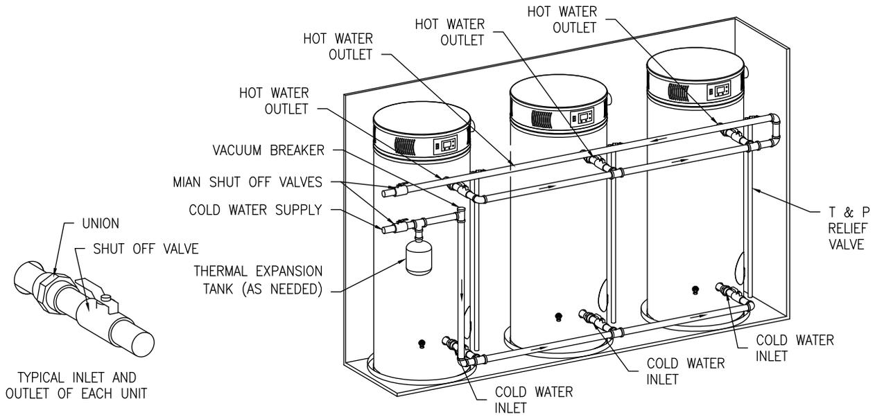
**Figure 7. Typical Three Water Heater Connection**
