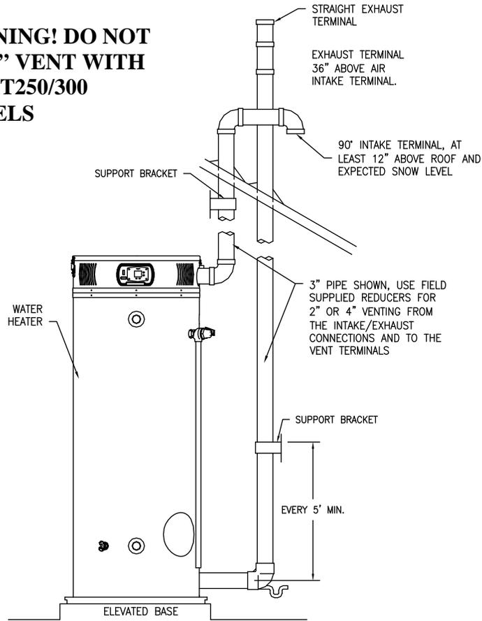
**Figure 13. Typical Vertical Direct Vent System Installation**
