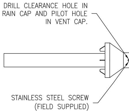
**Figure 21. Rain Cap to Small Vent Pipe Assembly**
