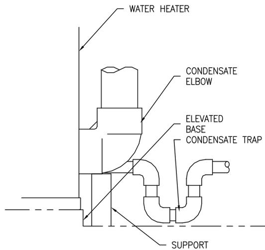
**Figure 2. Condensate Elbow With Trap**
