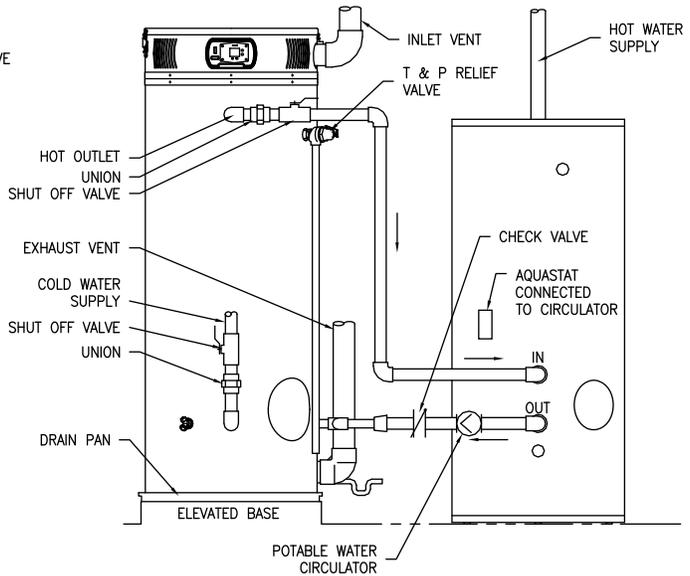
Figure 5. Typical Front Inlet Connect with Storage Heater
