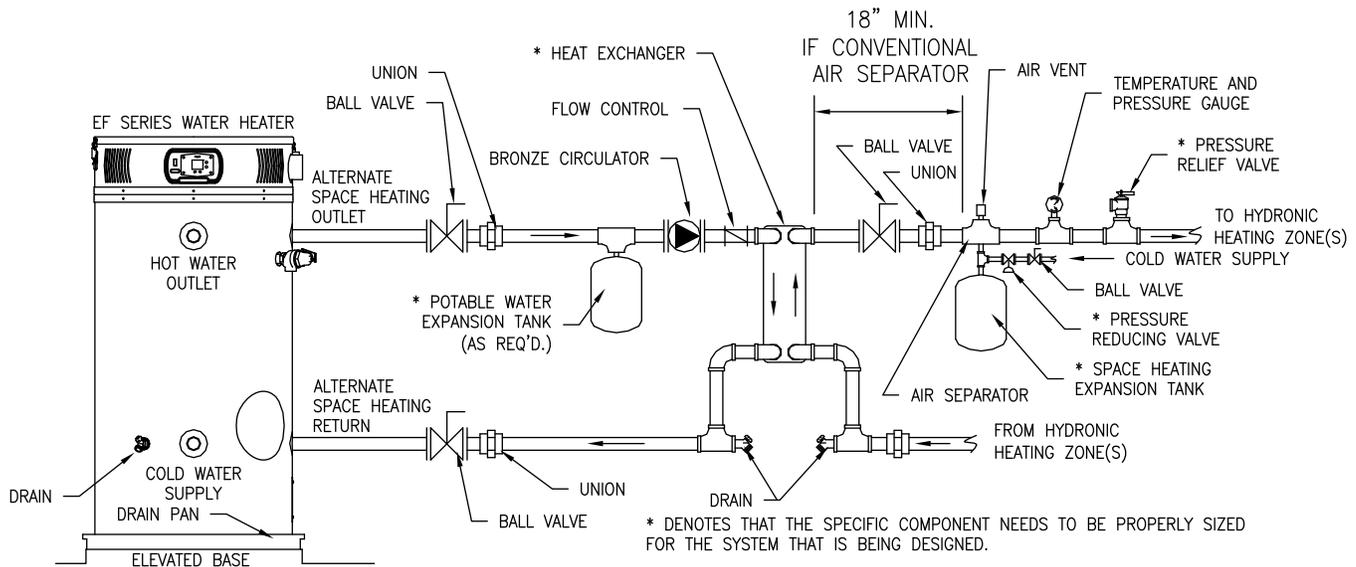
Figure 10. Typical Plumbing Schematic for Zoned Heating
