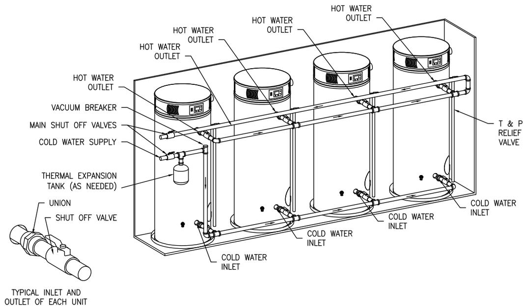
**Figure 8. Typical Four Water Heater Connection**
