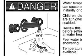
Water temperature over 125°F can cause severe burns instantly or death from scalds.
