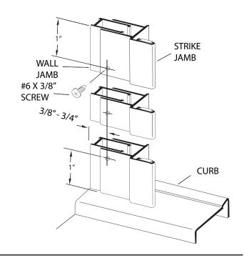
Slide the Hinge Jamb of the door panel assembly [**B**] over the mounted wall jambso the door will open outward. Adjust the door panel assembly so there is a 1/4" clearance between the strike jamb and the strike edge of the glass door with it being in the closed position.
