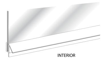
11 Place the sweep onto the bottom of the door. Stand inside the shower, close the door and mark the deflector part of the sweep at the inside edge of the strike jamb.
