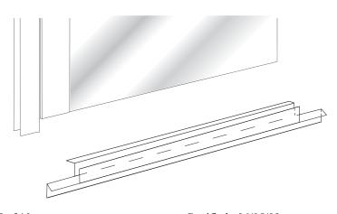
11 Align the clear bottom sweep to the bottom of the door with the deflector lip on the inside of the shower door. Mark the strike side of the bottom sweep even with the strike edge of the door.
