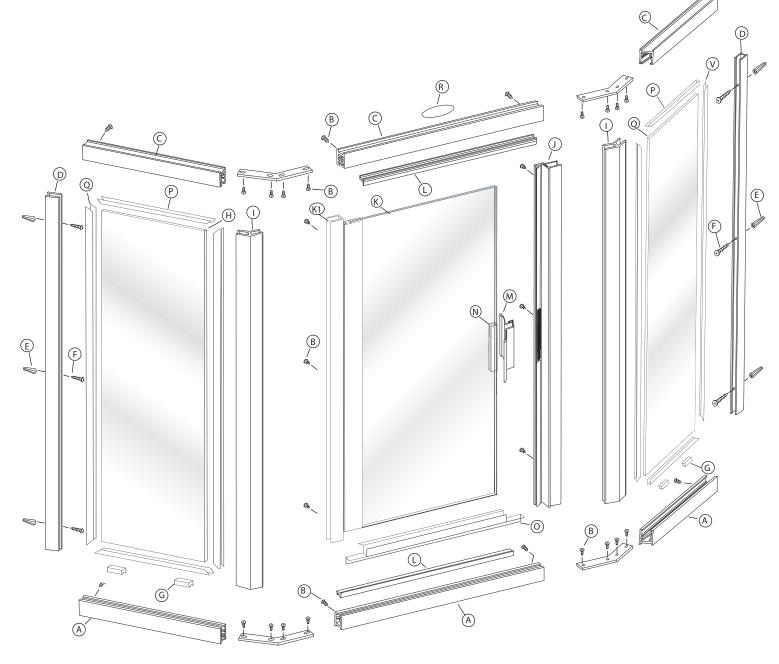
**1** The Semi-Frameless Continuous Hinge Shower door panel is completely reversible and may be installed hinge right or hinge left. For maximum waterproofing, the door should hinge off of the panel opposite the shower head wall. (see illustration) Careful as to not follow the illustrations exactly.
