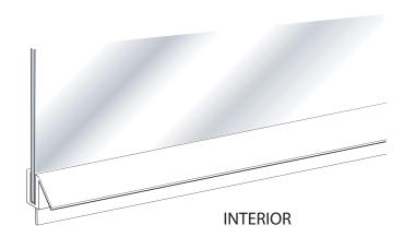
14 Place the sweep back onto the bottom of the door. Step inside the shower and close the door. Mark on the sweep at the edge of the strike jamb.
