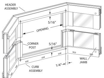
**NOTE:** If the Quick N' Stall option was selected, put the header in place and press down until it snaps over the vinyl. **9** Slide the strike jamb [**J**] over one of the corner posts. Be sure that the magnet is facing the exterior. Use a piece of tape to temporarily hold it in place.
