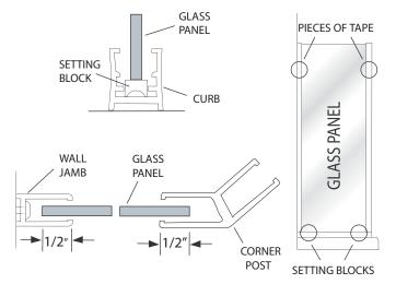
**NOTE:** If the Quick N' Stall option was selected, the setting blocks are not used. Set the glass panel in place and press down until it snaps into the curb.
